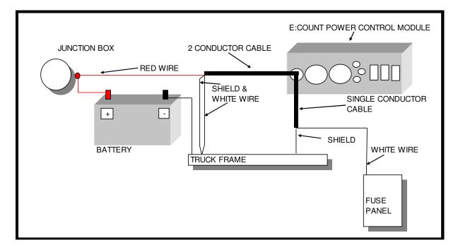
The power cable assembly consists of a **two conductor shielded** cable for power and a single conductor shielded cable for ignition pick-up. The two conductor cable should be routed to the vicinity of the truck battery and the single conductor cable to the vicinity of the fuse panel.
