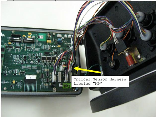
Figure 7. E:Count Optical Sensor Harness Connection
