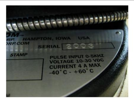
If the E:Count MCR-05 Serial Number stamped on the MID:COM Nameplate is greater than 2000 the RTD Digital Temperature Probe is installed.
