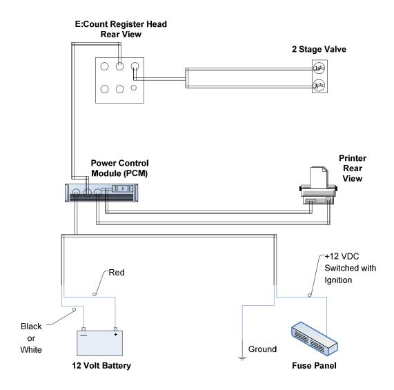
[MCR-09 LT: The Power Control Module is not used by the E:Count LT MCR-09.]
