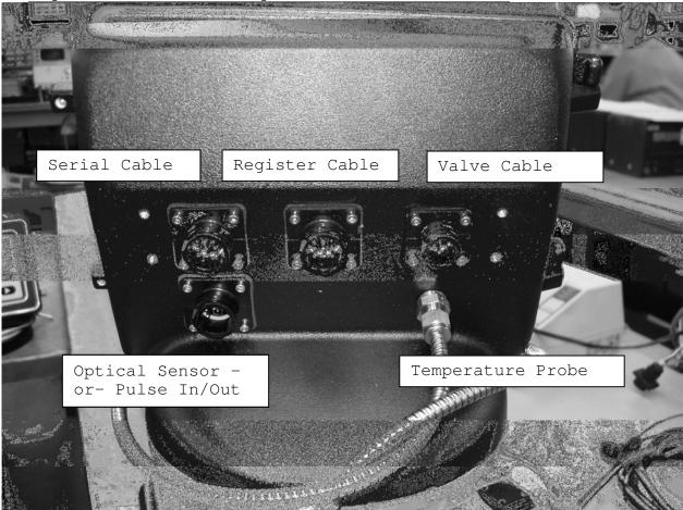
Figure 16. E:Count Register Cable Connections
