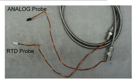
Figure 24. E:Count Temperature Probes
